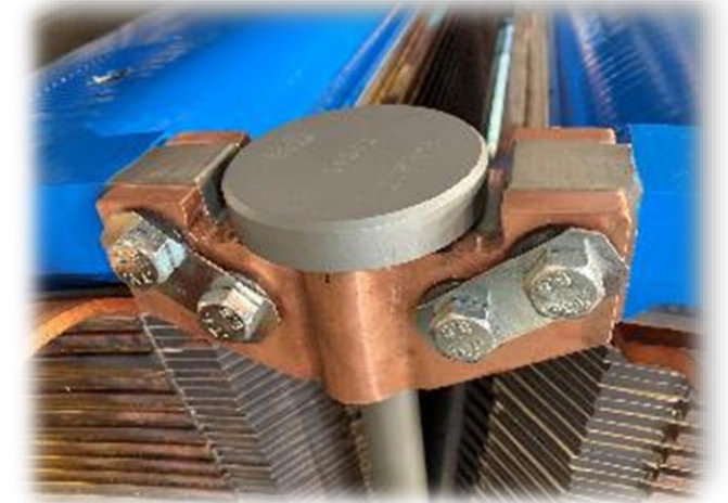
ANDRITZ damper winding design: very robust, integrated, interconnected
