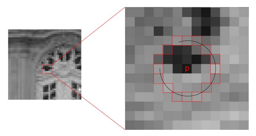
Count the number N of contiguos pixels around a center pixel p that are brighter than the center pixel. If N >= than some threshold this point is a feature location.
