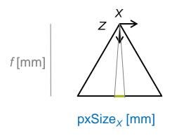
$GSD_X[m]$ focal length f[mm]depth Z[m] (= height h[m] for nadir camera)  $pxSize_X[mm]$
