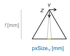
$GSD_{\gamma}[m]$ focal length f[mm]depth Z[m] (= height h[m] for nadir camera)  $pxSize_{\gamma}[mm]$
