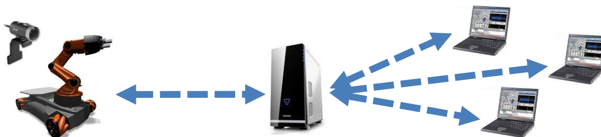
Fig. 1.: Setup of a remote experiment: Lab equipment <-> LabServer <-> User
