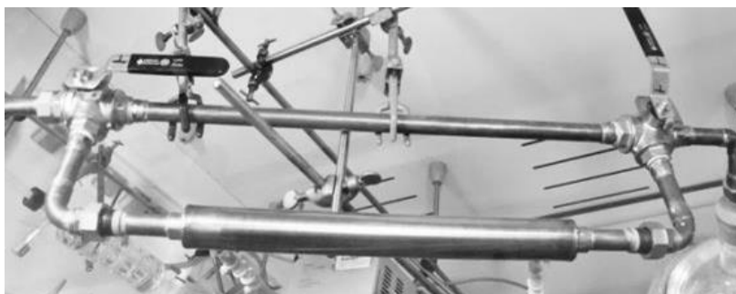
Fig.5: The „Löffler fork“: optional bypass of common lyne arms realized with randomly packed column
