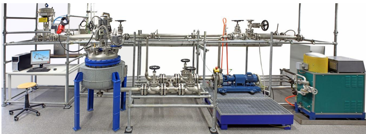
Fig. 2.: Remote setup of packed bed tube reactor for a catalysis process
